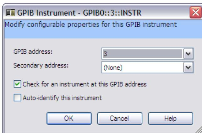
This example is for a connection to a Pegasus™/PC with a GPIB address of 3. This value may be different depending on how you configured the device. Note: *Auto-identify* should NOT be selected as neither the Pegasus™ nor LabMaster™ supports it.
