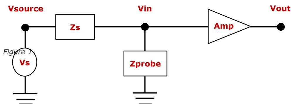
Figure 1 – simplified probe circuit
