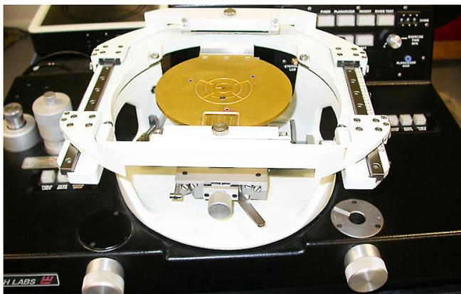
Compass chuck & probe card rails
